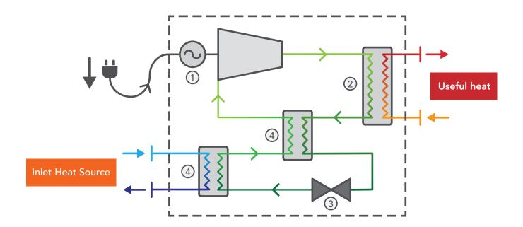
① Compressor The compressor suctions the working fluid and increases its pressure and temperature.
